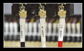
This special non-adhesive tape is made of a special material that is wound in the tape cassette as a flat tube. Once printed, the tube is opened up and passed over a cable or terminating connector. After heated with a heat gun, the tube will shrinks to about half its original width, and grips the cable.
