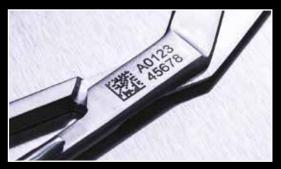
When printed, small holes are made in the tape which allows the etching chemical to permeate through the tape. An etching pad is placed over the tape and pushed onto the metallic item, an electrical circuit is completed. The metal then discolours and is permanently marked with serial numbers or other information.
