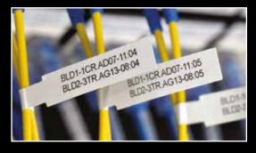
Suitable for cables with small diameter and ideal for fibre optic cable identification in the network industry. The label is a special pre-cut shape and once printed the long "tail" can be placed around the cable and the label simply folded over the tail to lock the label into position.
